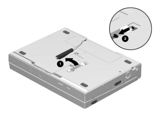
Figure 5-8. Removing the Auxiliary Battery
